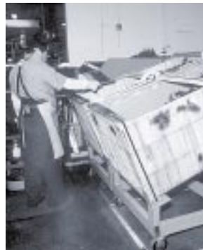
Tilted container with step for easier access
