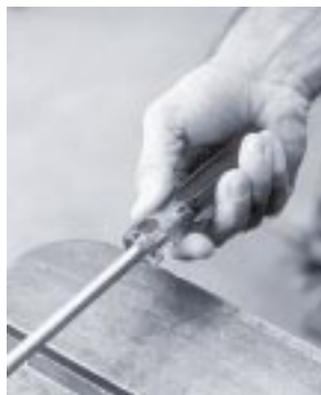
Tool handles digging into the palm and fingers
